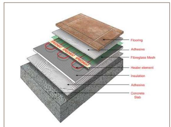
Different insulation material is suited for different floor surfaces and heating requirements, offering you a tailor made insulated floor heating system.
