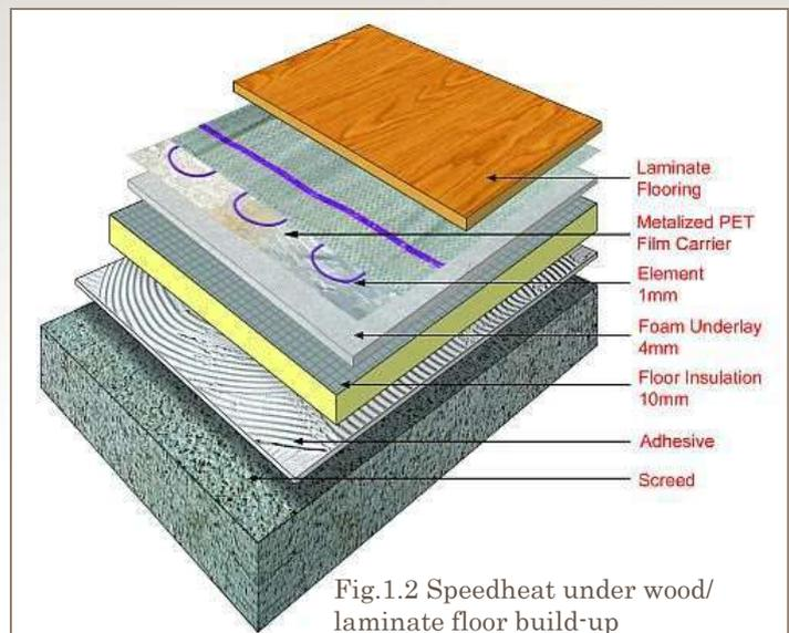
Fig.1.2 Speedheat under wood/laminate floor build-up
